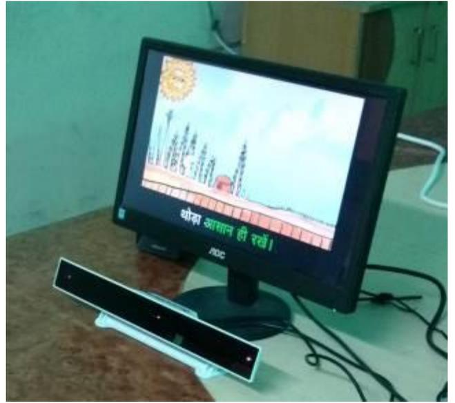
Computer set up with eye tracking device
